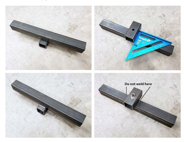
Secure the welded assembly to the main rails of the frame jig using one 1-1/2"x5" rectangle plate (clamp bar) with one 1/2"x 1-3/4" bolt (with a lock washer and washer). When the fixture is in its final position torque the bolt to 15 ft-lbs. Do not over-tighten or you will bend the clamp bar.
