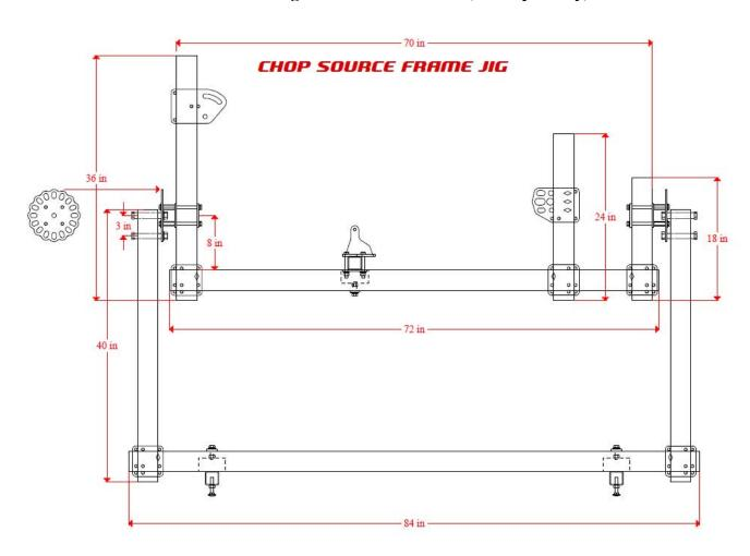
Full Motorcycle Frame Jig Kit (shown with adjustable width fixture, standard feet, and 3/4" threaded rods and spacer material)
