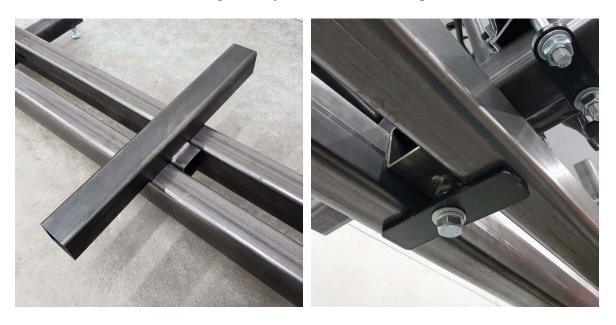
Finish the assembly by installing the fixture on the 2x2'' tube as shown below. When bolting the fixture to your frame, if needed, drill out the hole at the top of each bracket to fit your bolts. Since every frame is different, you will need to supply these bolts.
