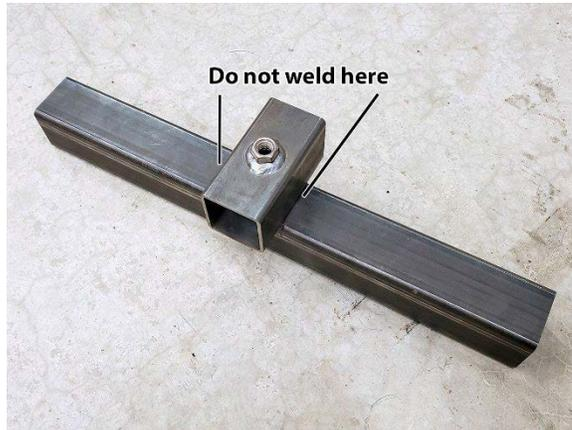
Secure the welded assembly to the main rails of the frame jig using one 1-1/2"x5" rectangle plate (clamp bar) with one 1/2" x 1-3/4" bolt (with a lock washer and washer).
