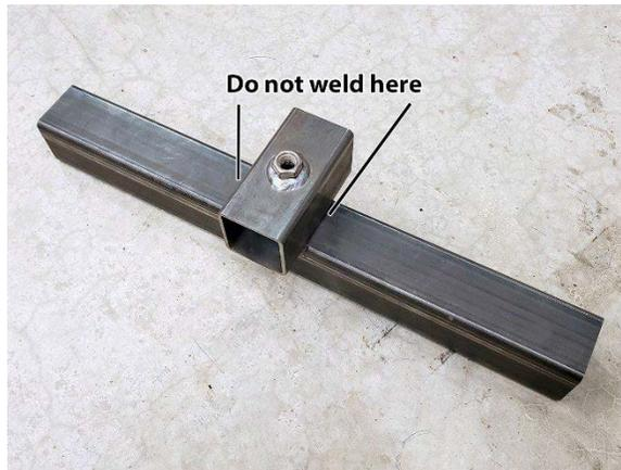
Secure the welded assembly to the main rails of the frame jig using one 1-1/2"x5" rectangle plate (clamp bar) with one 1/2" x 1-3/4" bolt (with a lock washer and washer). When the fixture is in its final position torque the bolt to 15 ft-lbs. Do not over-tighten or you will bend the clamp bar.
