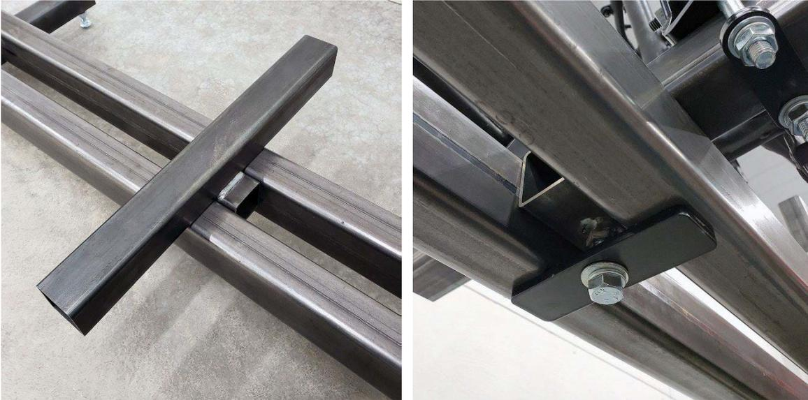
Finish the assembly by installing the fixture on the 2x2" tube as shown below. When bolting the fixture to your frame, if needed, drill out the hole at the top of each bracket to fit your bolts. Since every frame is different, you will need to supply these bolts.
