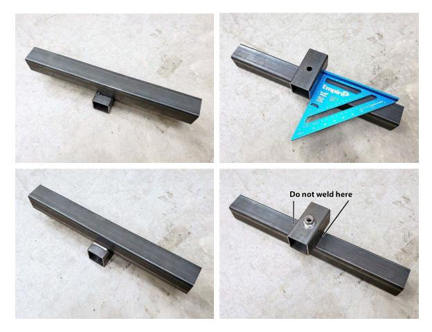
Secure the welded assembly to the main rails of the frame jig using one 1-1/2''x5'' rectangle plate (clamp bar) with one 1/2'' x 1-3/4'' bolt (with a lock washer and washer).
