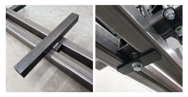
Finish the assembly by installing the fixture on the 2x2'' tube as shown below. The cones are held in place with a threaded rod, two washers, and two nuts. Wait to install the cones until you have a frame or bottom bracket to mount in the jig. **Do not overtighten the 3/4'' nuts.** They just need to be tight enough to make sure the bottom bracket doesn't move.
